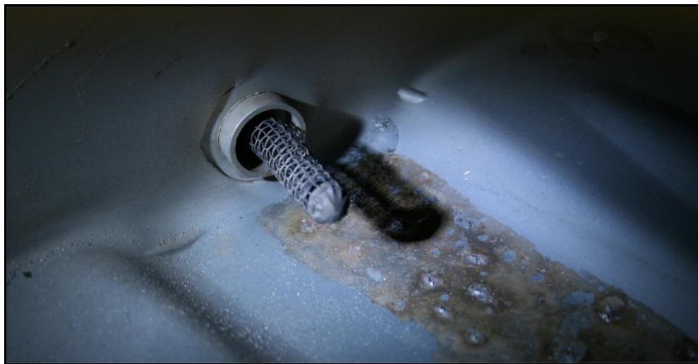
Photo No. 4: Internal filter in fuel tank outlet
